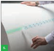
Figure 5 + 6: Remove the lower part of the liner from the tape before accelerating the reel.
