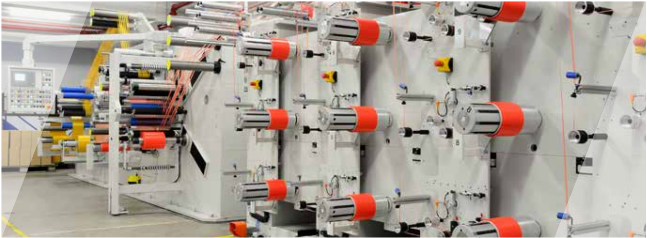
Running length spools for spool diameter 300 mm (max. 500 mm)
