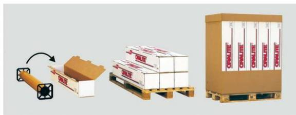
Rolls should be stored in the original carton. The rolls have standard spacers [core plug] that prevent contact between the roll surface and the carton and thus the formation of pressure marks and surface damage. Please make sure that partly processed rolls are never stored without spacers.
