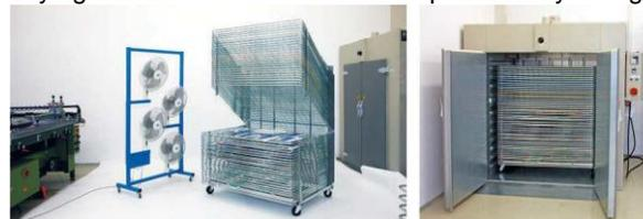
convection ovens. These closed systems permit a low-dust drying phase at constant temperature, low air humidity and do not subject the operator to solvent vapors. The following drying times are general guidelines:
