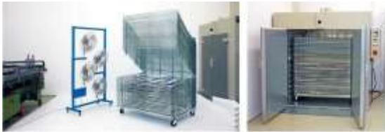
Drying conditions can be further optimized by using convection ovens. These closed systems permit a low-dust drying phase at constant temperature, low air humidity and do not subject the operator to solvent vapours.
