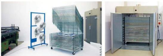
Drying conditions can be further optimised by using convection ovens. These closed systems permit a low-dust drying phase at constant temperature, low air humidity and do not subject the operator to solvent vapours.
