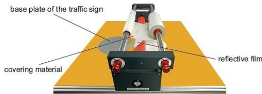
When several film webs need to be bonded side by side, these should always overlap. Depending on the format, the overlap should be 3-5 mm.
