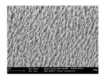
The directly created PlasmAR®-strukture (PAR) can be applied to plano curved as well as microstructured surfaces. It is possible to structure different polymers up to a size of 940 mm in diameter (37").
