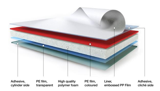
The **ORAFLEX**® Cushion Tapes' compressible foam and film reinforcement construction technology guarantees an optimized thickness accuracy, with minimal thickness tolerances (+/- 0.02 mm).
